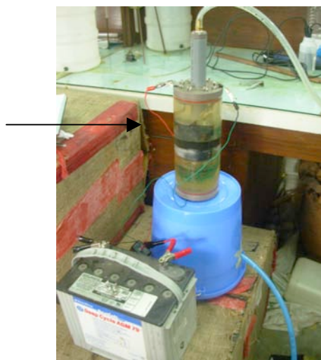
Figure 3: ECAR prototype device (shown by arrow) being tested at Bangladesh University of Engineering and Technology (BUET), in Dhaka, Bangladesh. Notice the 12V car battery - in the field, batteries could be coupled with solar photovoltaic panels.
