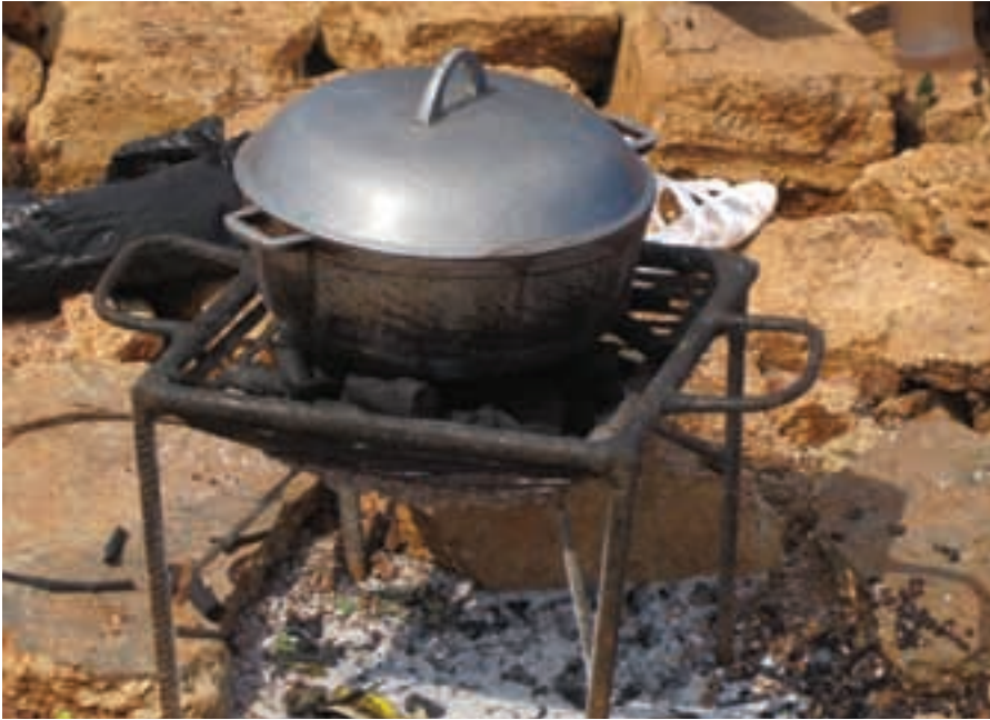
Figure 2: Pot on stove made of Rebar (Source: Kayje Booker)
