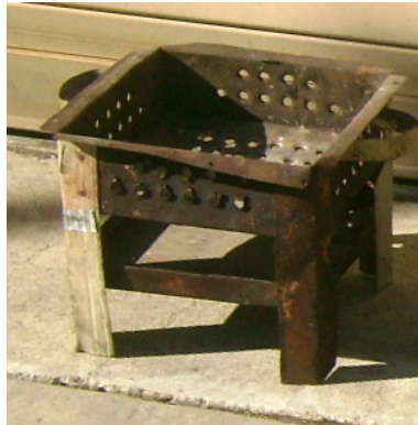
Figure 1: Traditional Haitian stove: height: 27 cm; length/width: 11 cm; and weight: 2.8 kg.
