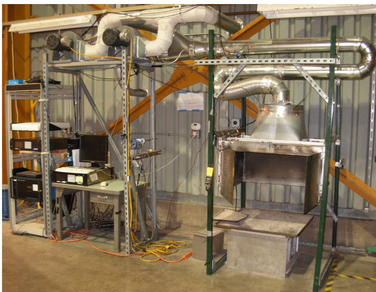
Figure 5: The stove testing system at LBNL. The exhaust hood and ductwork are seen on the right-hand portion of the photo; the instrumentation is on the left.
